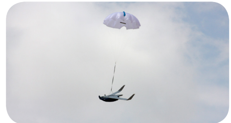
The APEX launches with a catapult system and lands using a parachute system for easy recovery
